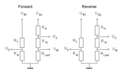
The resistors  $R_H$  and  $R_T$  are located on the thin film element. All further resistors are on the hybrid.
